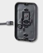
With the quick connect wiring harness, you no longer have to juggle a reader while wiring it to the controller wires. Once the wires are connected, you simply plug the wiring harness into the back of the reader. An internal gasket creates a tight seal, preventing water and dust from entering the reader.
