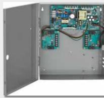
Schlage and Von Duprin power supplies feature a flat mounting design and polarized locking connectors for option boards. This design eliminates the need for racks and side connectors, and provides easier access to the terminal blocks for connection of peripheral devices including strikes, electromagnetic locks and card readers.
